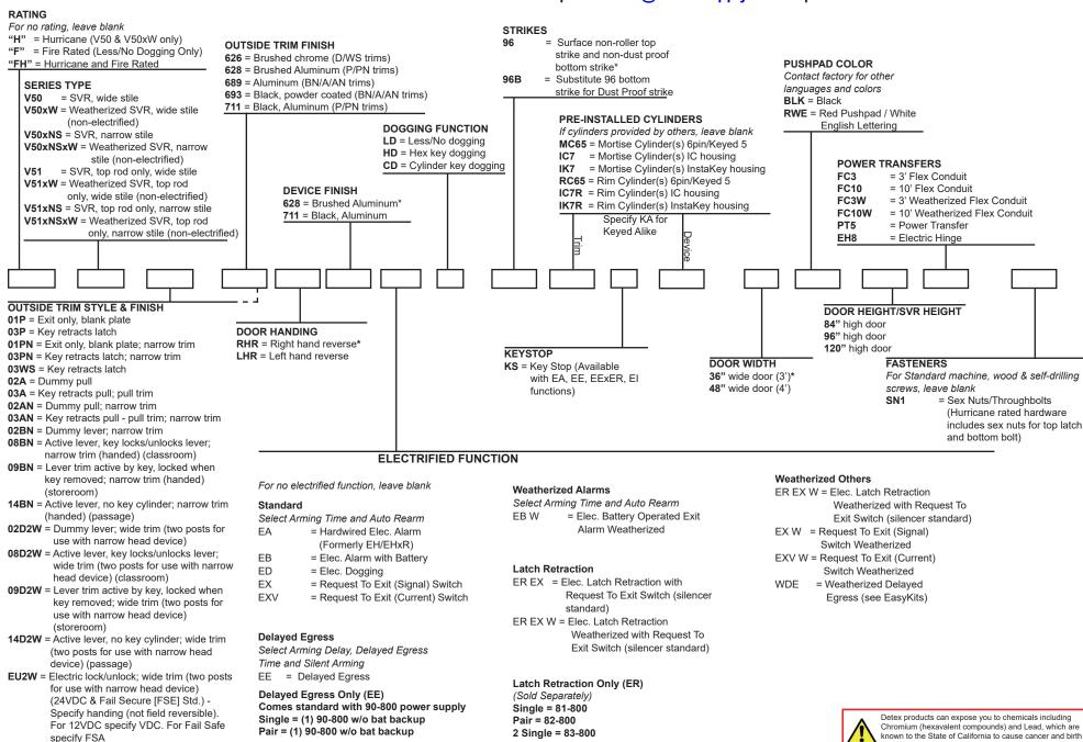
Fire-rated trims must be Fail Safe (FSA)
